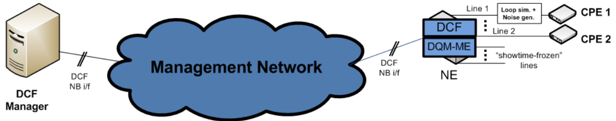
Figure 4 – Test Configuration for performance tests - Distributed DCF in the NE
