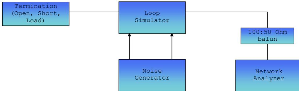
NOTE - The unbalanced side of the balun might be of other impedances than 50 Ohm, as long as it matches the network analyzer
